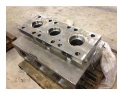
**Result:** After nine months, all surfaces coated with **HT 365** were rust-free, especially in the threaded areas. This result preserves the functionality of the block and value for eventual resale.
