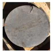
After 90 days, Sample A was observed for the second time and had just begun to show signs of rust bloom on the sides that were treated with HT
